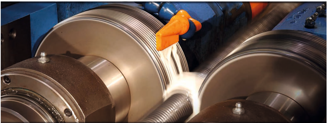
Pic – Rolling of Grip Bolts in a Circular rolling machine.
