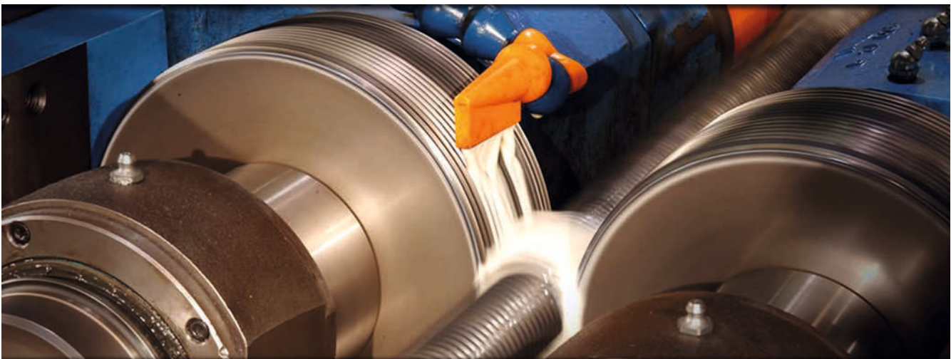
Pic – Rolling of Grip Bolts in a Circular rolling machine.
